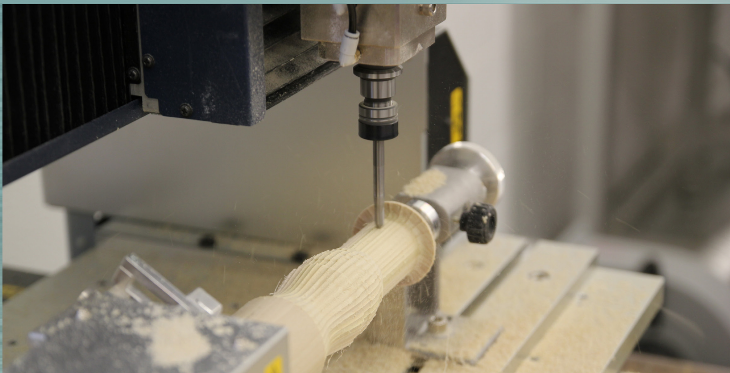
Advanced technologies such as this Roland benchtop milling machine allow students to fabricate CAD/CAM projects.
