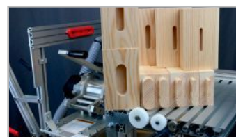
Mortise and tenon sizes are changed by using different guide bearings and bits.
